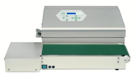
the sealer. The adjustable hand feed chute sets the seal height of the seal in relation to the top of the pack. Poly H is a fixed speed machine which allows the controls to be kept to a minimum, incorporating a power switch and a precise digital adjustable temperature controller to produce a consistent high-quality seal.
